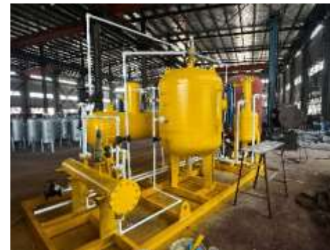
重整工艺空冷器间接喷雾降温 Indirect spray cooling for the air cooler in reformer unit
