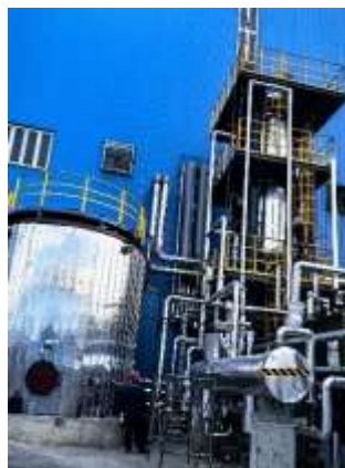
煤焦油减压闪蒸深度脱水 Remove water from coal tar oil by vacuum distillation
