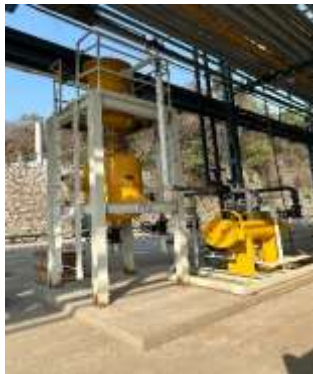
电脱盐污水旋流除油、除油泥 Remove oil and sludge from crude oil desalting water
